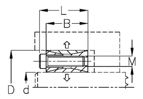
$\begin{array}{lll} \text{B mm} & = 24 \\ \text{d H8 mm} & = 55 \\ \text{D mm} & = 85 \\ \text{Fit tolerance} & = \text{Aksel k11-h11, Nav N11-H11} \\ \text{F kN torque} & = 51.6 \\ \text{L mm} & = 32 \\ \text{M mm} & = \text{M8} \\ \text{P N/mm2 surface pressure on shaft/hub} = 48 \end{array}$
